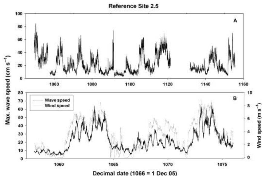
**Fig. 3** (A) A 106-day record of maximum wave speed at Reference Site 2.5 between November 2005 and February 2006. (B) A shorter-term (41 days) record of wave and local wind speed extracted from A illustrating tight coupling of local wind and maximum wave speeds.
