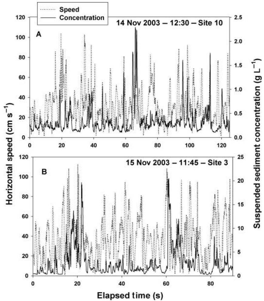
Fig. 8 Representative portions of high-frequency (10 Hz) measurements of horizontal speed measured using the ADV and suspended sediment concentration measured using the optical backscatter sensor collected at two sites in November 2003.
