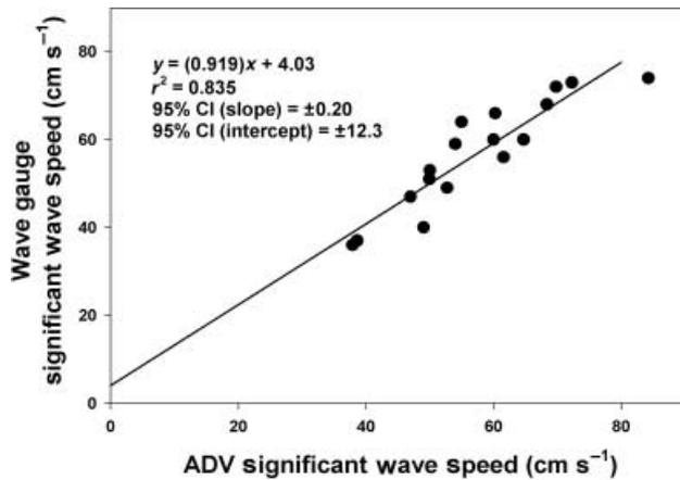
**Fig. 2** Comparison of significant wave speed calculated from high-frequency pressure records to that measured directly and simultaneously using an ADV located  $\approx 1$  m away. Data points were obtained between 13 and 17 November 2003 among five sites distributed along the beach (within Sites 1, 2, 3, and 10 and at the boundary between Sites 7 and 8). CI – statistical confidence interval of slope or intercept.
