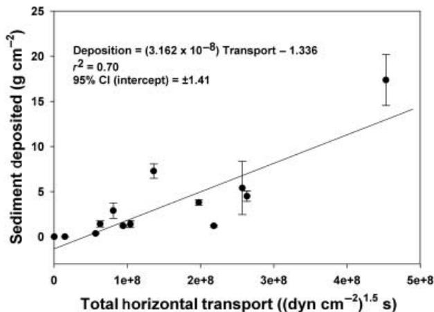
Fig. 9 Sediment accumulated in traps as a function of the total (time-integrated) horizontal transport predicted for the period of trap deployment at the location of each measurement. CI – statistical confidence interval of intercept.
