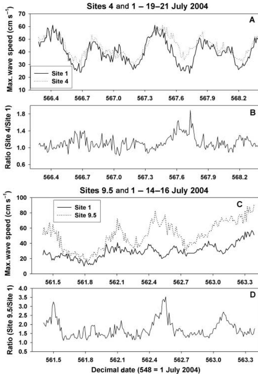
**Fig. 4** Short-term records comparing maximum wave speeds at two locations along the beach. (A) Maximum wave speeds at Sites 4 and 1 on 19–21 July 2004. (B) Ratio of two speeds. (C) Maximum wave speeds at Site 9.5 and 1 on 14–16 July 2004. (D) Ratio of two speeds.
