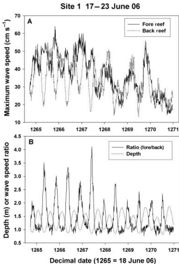
Fig. 7 (A) Maximum wave speeds calculated seaward (Fore Reef) and landward (Back Reef) of the fringing platform reef at Reference Site 1 between 17 and 23 June 2006. (B) Ratio of wave speeds relative to tidal stage (depth).
